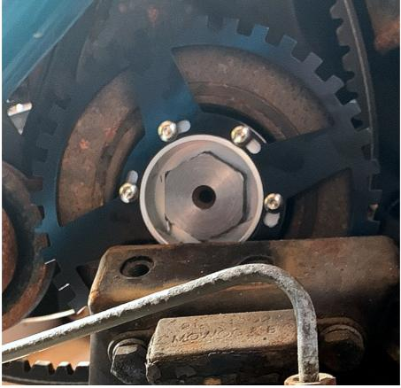
**Step 6:**Please align the gap with the trigger wheel
