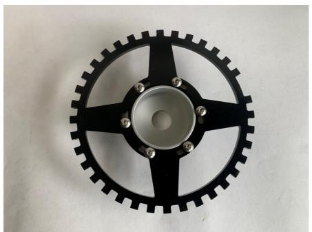
**Step 5:**Install the trigger wheel assembly onto the pulley wheel
