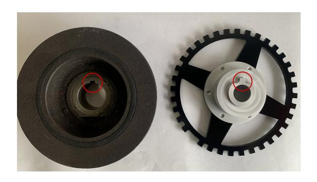
**Step 7:**After trigger wheel installation, loosen the screws to align the sensor with the trigger wheel
